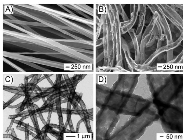
**Figure 2.** A,B) SEM images of PLA nanofibers and PPy nanotubes, respectively. C,D) TEM images of the PPy nanotubes. The PPy nanotubes were produced by soaking the PLA-PPy core–sheath nanofibers in DCM to selectively remove the PLA cores. The polymerization was conducted with  $\text{Fe}^{3+}$  as an oxidant and  $\text{Cl}^-$  as a dopant.
