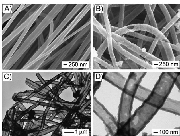
**Figure 1.** A,B) SEM images of PCL nanofibers and PPy nanotubes, respectively. C,D) TEM images of the PPy nanotubes. The nanotubes were obtained by soaking the PCL-PPy core–sheath nanofibers in DCM to selectively remove the cores. The polymerization was conducted with  $\text{Fe}^{3+}$  as an oxidant and  $\text{Cl}^-$  as a dopant.
