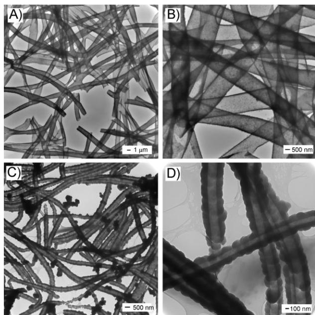
**Figure 3.** TEM images of PPy nanotubes prepared using APS as an oxidant and PTSA as a dopant, while PCL (A,B) and PLA (C,D) nanofibers served as the templates, respectively. For polymerization, the PPy nanotubes were obtained by soaking the core-sheath nanofibers in DCM to selectively remove the cores.
